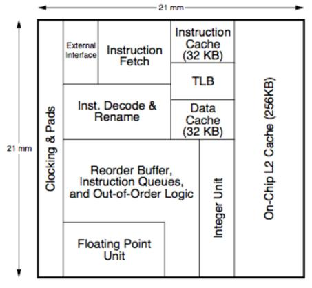
Figure 2. Floorplan for the six-issue dynamic superscalar microprocessor.
