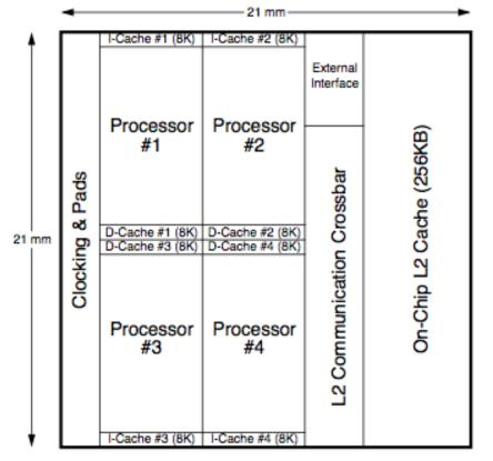
Figure 3. Floorplan for the four-way single-chip multiprocessor.
